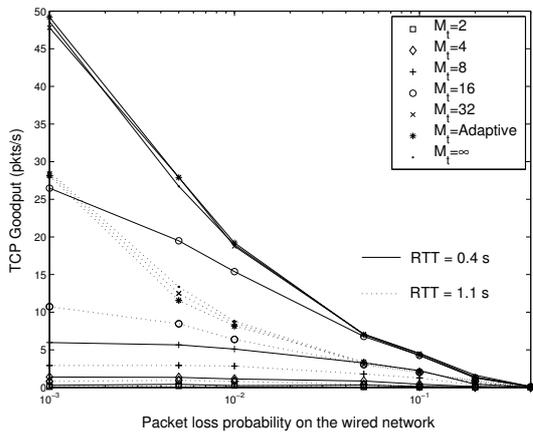
Figure 6: TCP Goodput varying  $p_f$  for 1 TCP Source.
