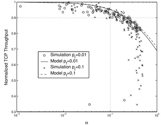
Figure 5: Normalized TCP Throughput vs packet loss degree,  $\alpha$ , in the wireless link (RTT=1.1s).
