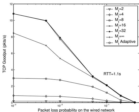
Figure 7: TCP Goodput varying  $p_f$  for 8 TCP Sources.
