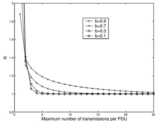
Figure 8:  $\mathcal{R}$  varying the maximum number of transmission per PDU.
